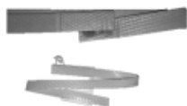
Strapping band: Top: closed- band still circular Bottom: open- band has been cut
